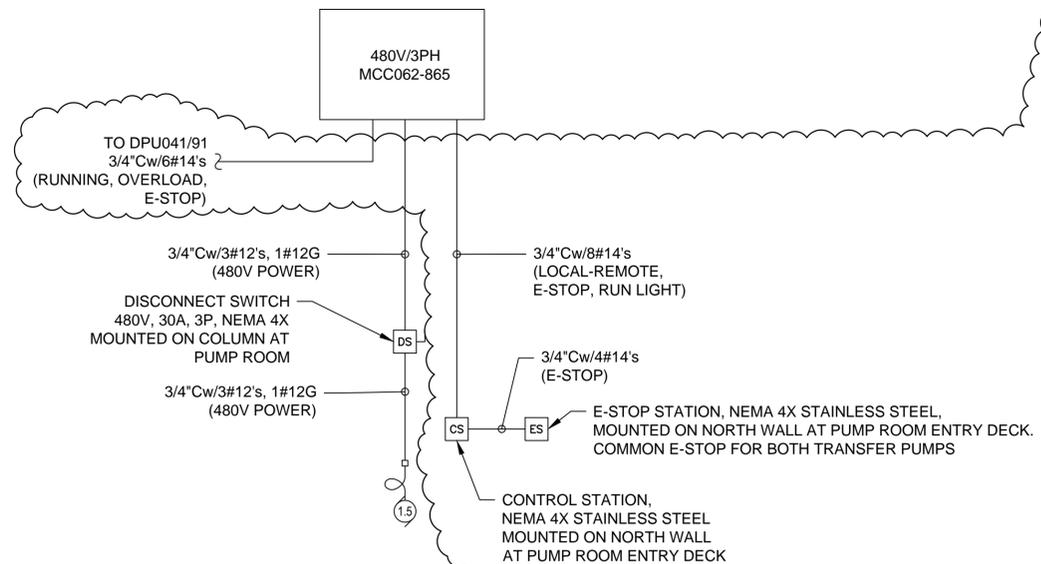
**SODIUM HYPOCHLORITE TRANSFER PUMPS WIRING SCHEMATIC**
