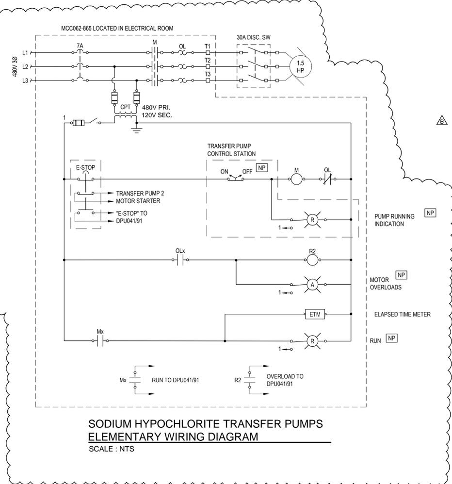
**SODIUM HYPOCHLORITE TRANSFER PUMPS ELEMENTARY WIRING DIAGRAM**
