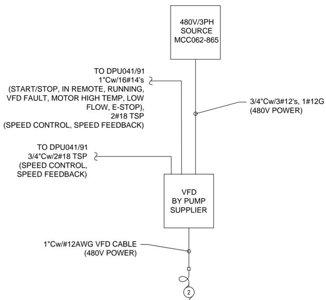
**SODIUM HYPOCHLORITE FEED PUMPS WIRING SCHEMATIC**
