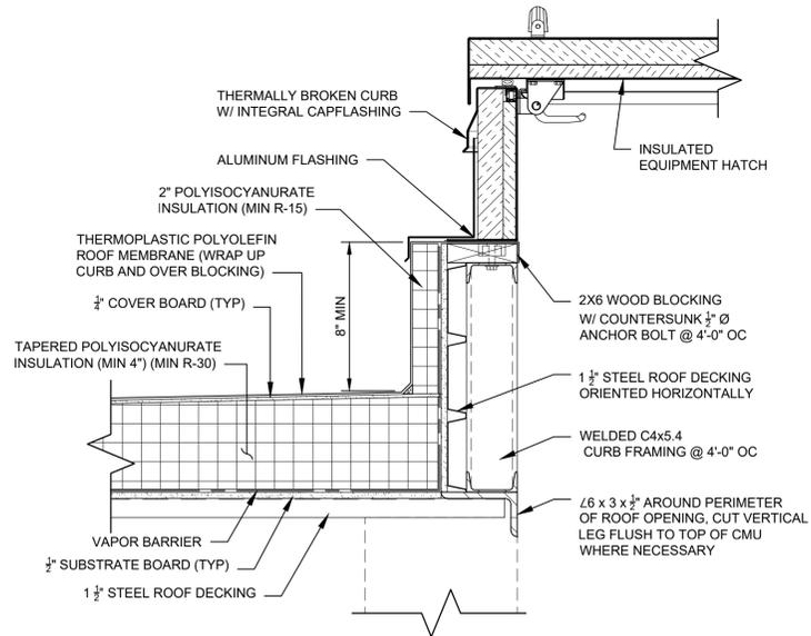
**ROOF HATCH CURB DETAIL**
