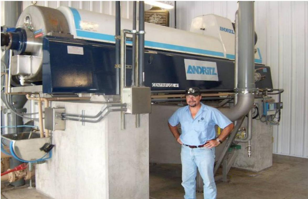
The IN-LINE design of our ANDRITZ decanter centrifuges reduces the floor space requirements to a minimum. Its isostatic design minimizes vibrations and noise level.
