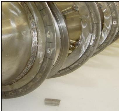
Field replaceable sintered tungsten carbide tiles the entire length of the scroll
