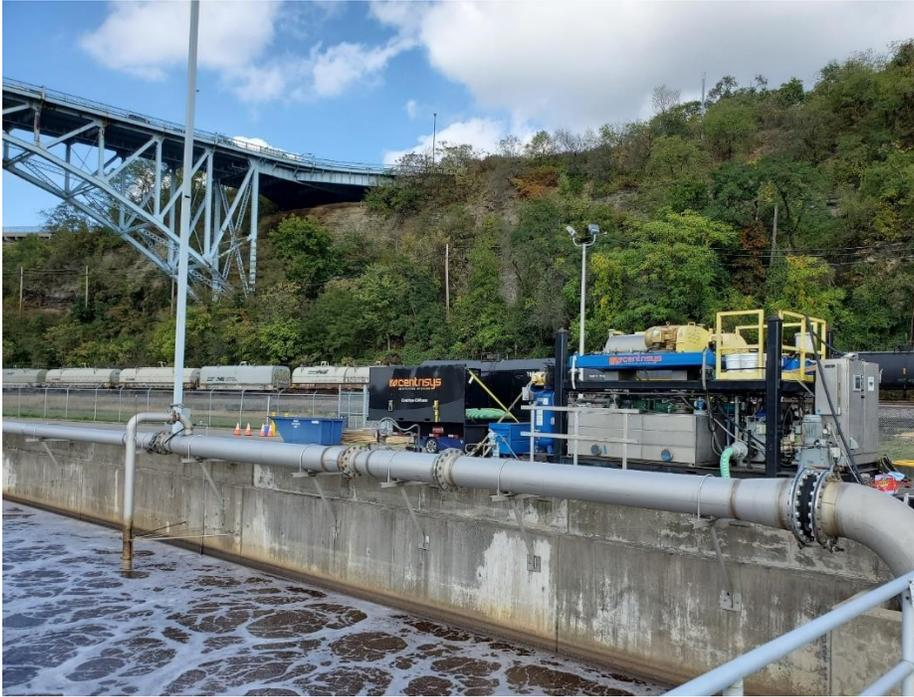
**Figure 3.** Sample collection side of THK200 skid trailer.
