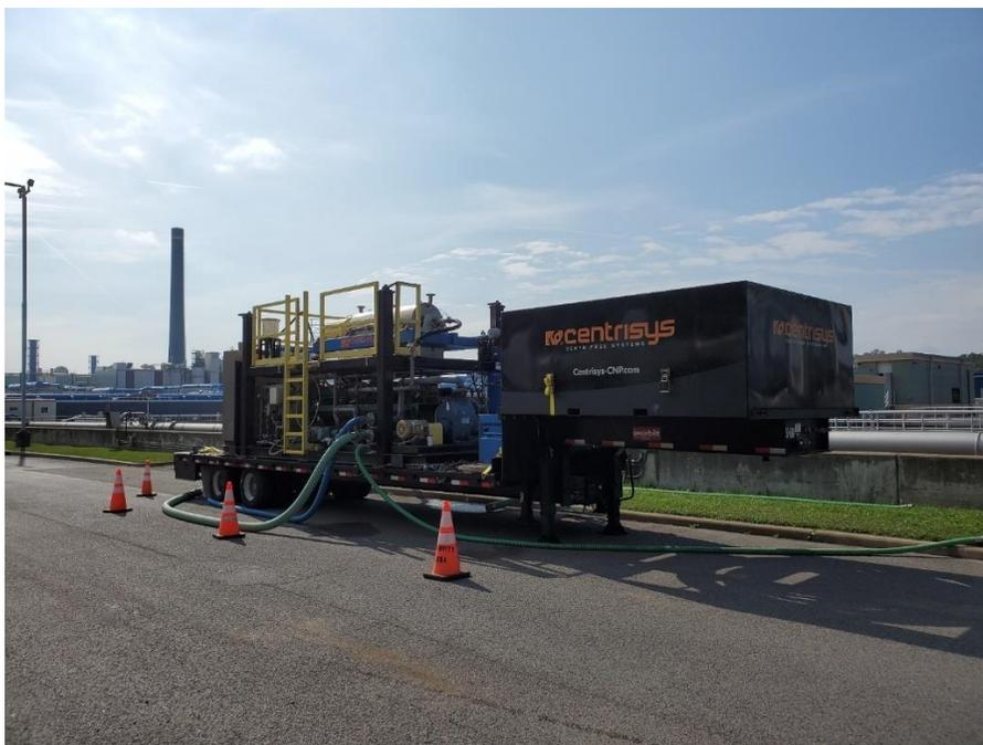
**Figure 2.** Trailer mounted Centrisys THK200 thickening centrifuge skid.
