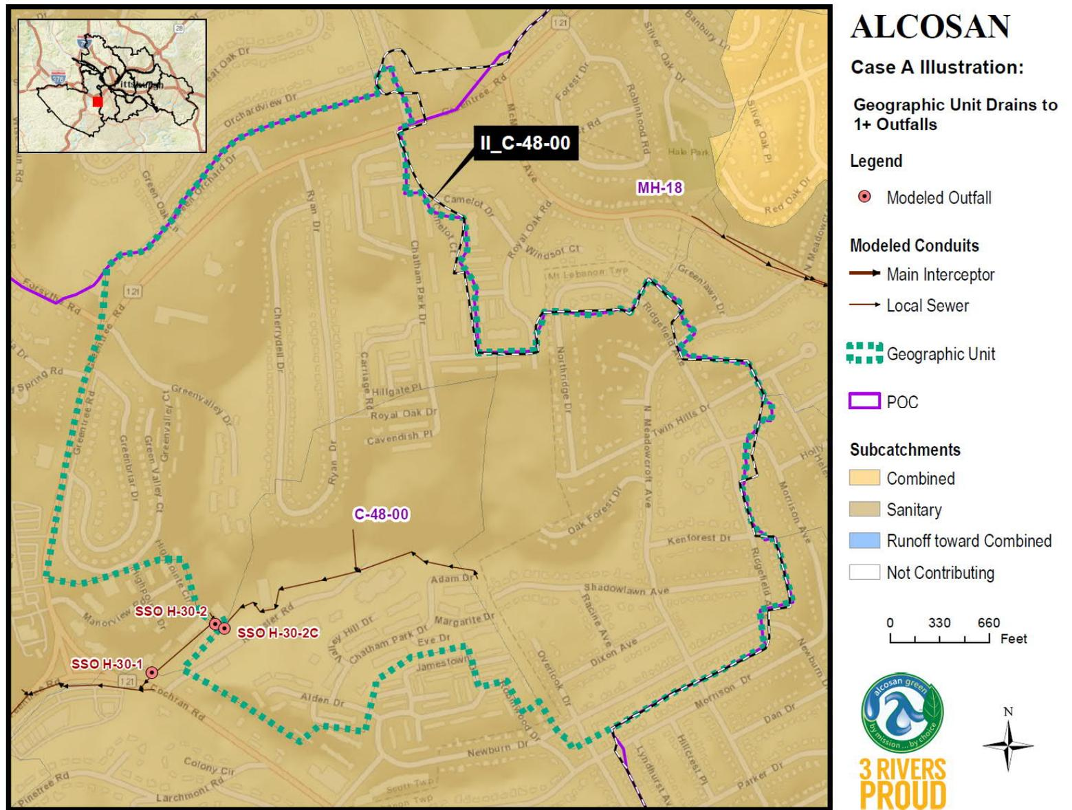
Figure 1. Case A Illustration: Geographic Unit Drains to 1+ Outfalls
