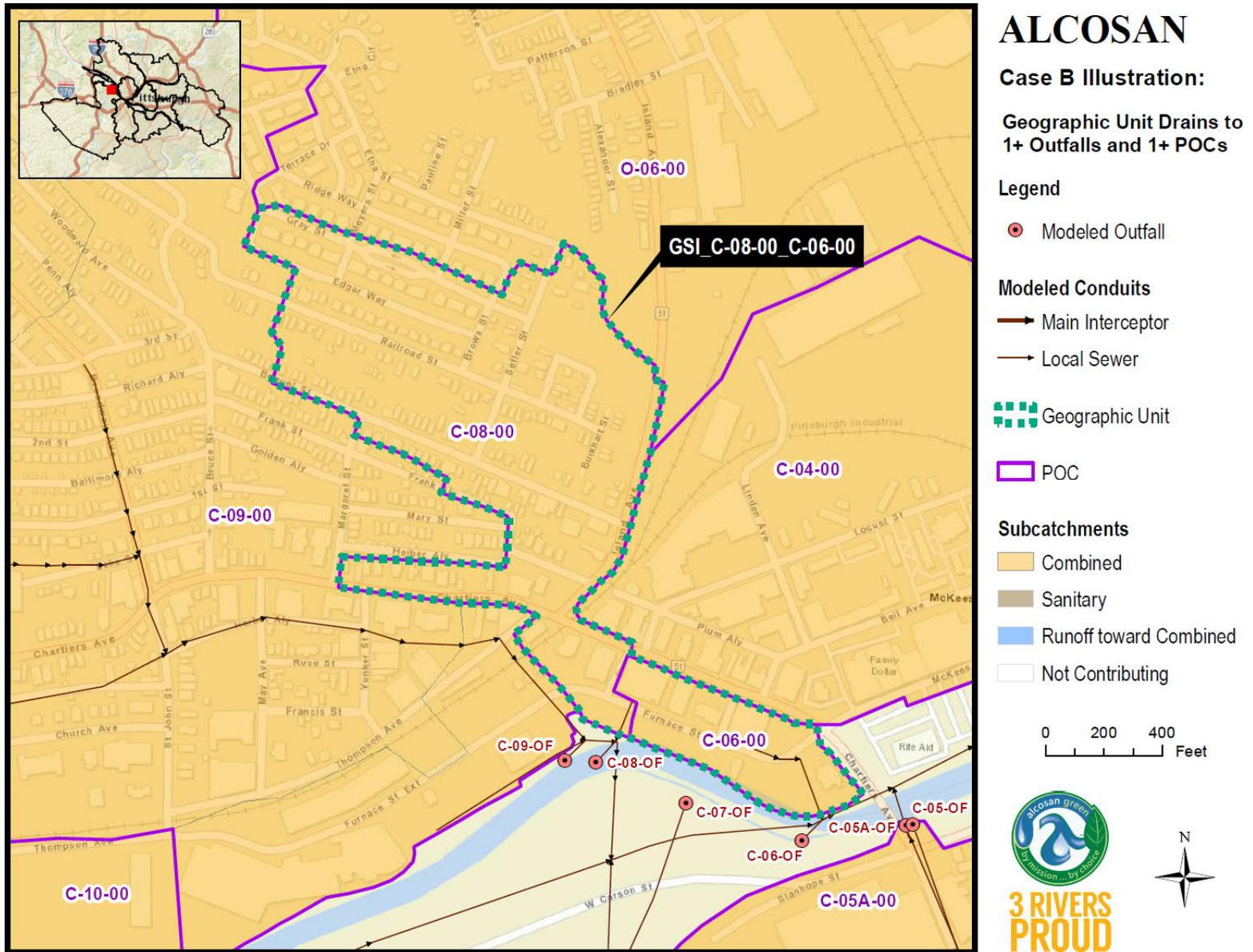
Figure 2. Case B Illustration: Geographic Unit Drains to 1+ Outfalls and 1+ POCs
