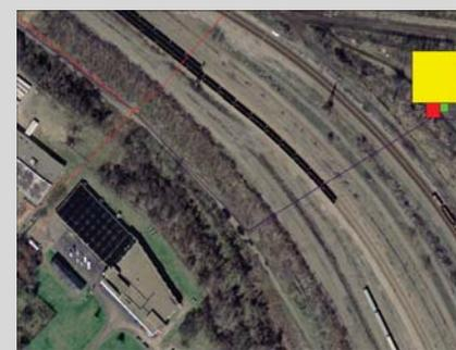
Retention Treatment Basins (RTBs) are one of the proposed technologies for the control of CSOs within the LOGR Planning Basin. The overflows from the existing CSO outfalls would be directed to these RTBs where the CSOs would be treated by screening and disinfecting the flow prior to discharge to the Ohio River. The above graphic shows a potential layout of an RTB to control the CSOs within Stowe Township.
