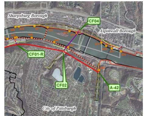
**ALCOSAN is evaluating the installation of a tunnel as a regional based alternative. One of the tunnel scenarios being evaluated would extend a tunnel to the A-42 CSO located near Washington Boulevard in Pittsburgh. This CSO is the largest (by volume) in the ALCOSAN service area. Addressing this large overflow will be an important component of the Upper Allegheny Basin's Facility Plan.**
