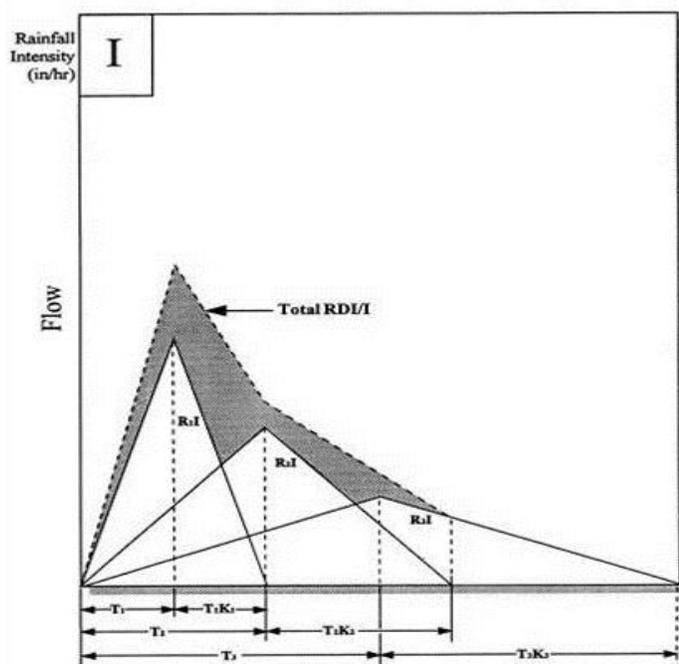
**Figure 4-12: Three triangular unit hydrographs used in the H&H models to represent the sewer system response to a storm event**
