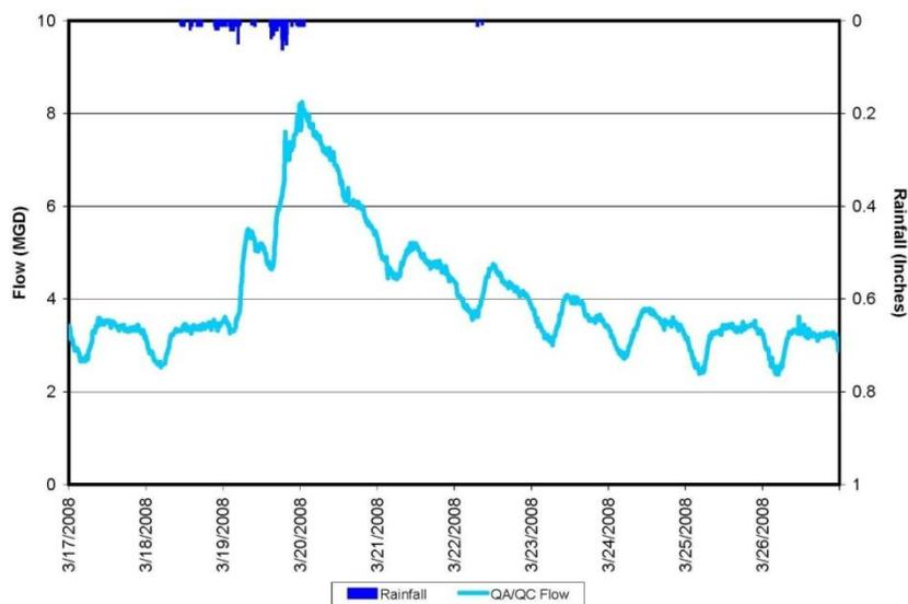
Figure 4-11: Example of a monitored sewer system response to a storm event showing typical storm peak and recession limb
