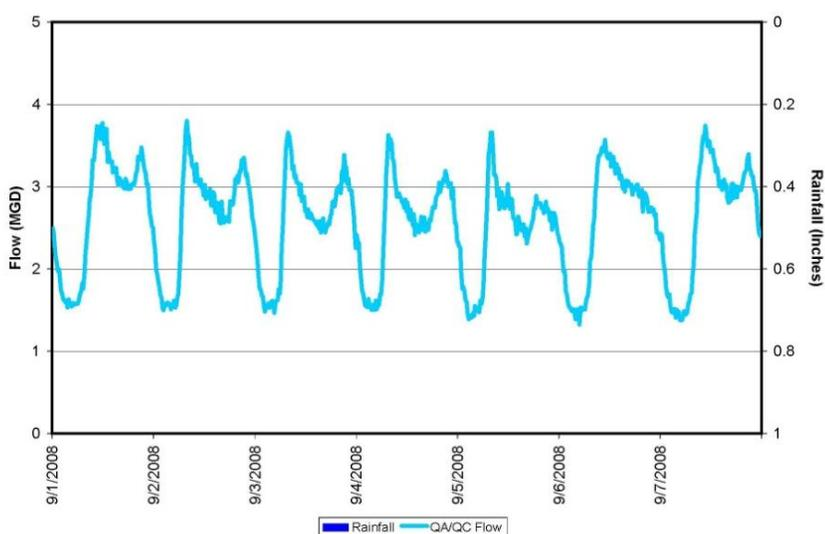
**Figure 4-10: Example of monitored dry weather wastewater flow from a residential area with typical diurnal week-day, weekend**
