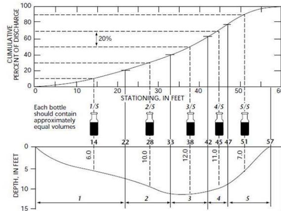
A single vertical (SV), depth-integrated, isokinetic sample involves lowering the sampler at a predetermined constant transit rate until slight contact is made with the streambed. Upon contacting the streambed, the sampler is immediately raised at the same constant transit rate until the sampler completes the vertical traverse.
