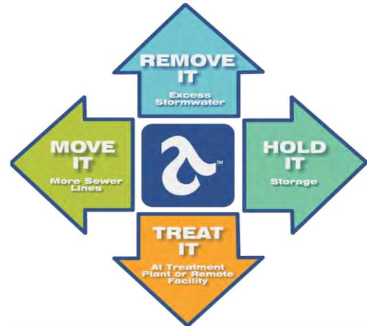
*Figure 1-1: Four Categories of Sewer Overflow Control Technologies*
