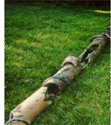
*Figure 6-4: Deteriorated Building Lateral Sewer*
