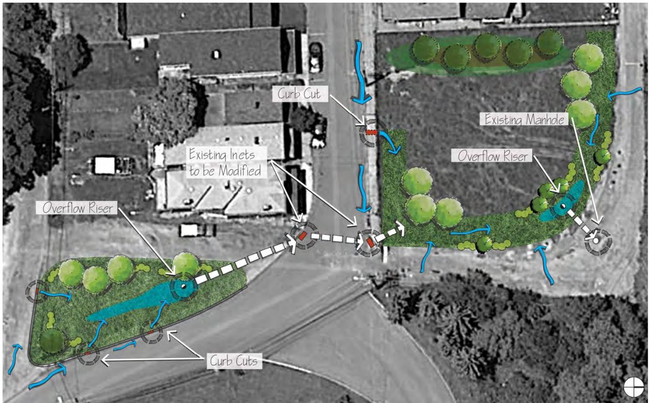
*Figure 4-27: Fleming Avenue GSI Concept Plan*
