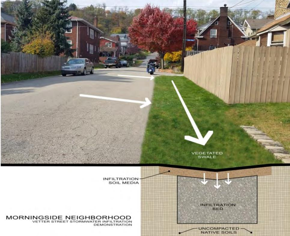
*Figure 4-23: Morningside Infiltration Trench Rendering*
