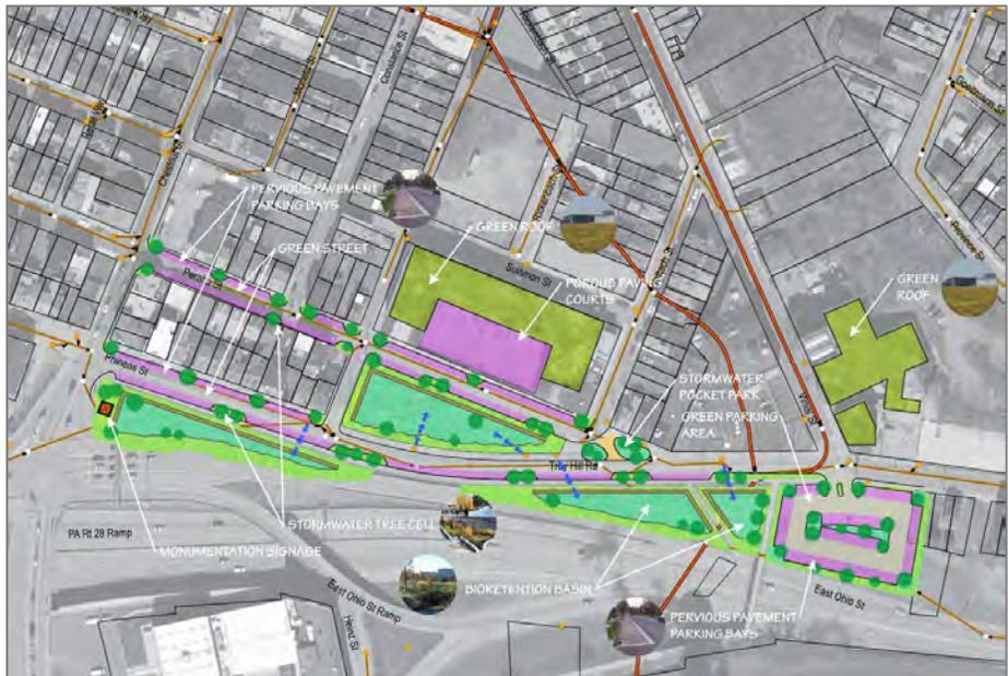
*Figure 4-5: Spring Garden Green Stormwater Infrastructure Concept Design*
