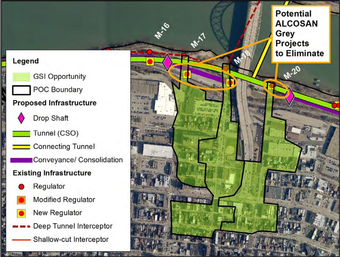
*Figure 3-24: Example of Evaluating Opportunities to Eliminate Grey Projects with GSI for Outfalls M-17, M-18 and M-20*
