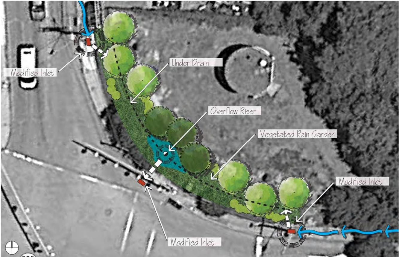
*Figure 4-26: ALCOSAN Access Shaft M-30 GSI Concept Plan*
