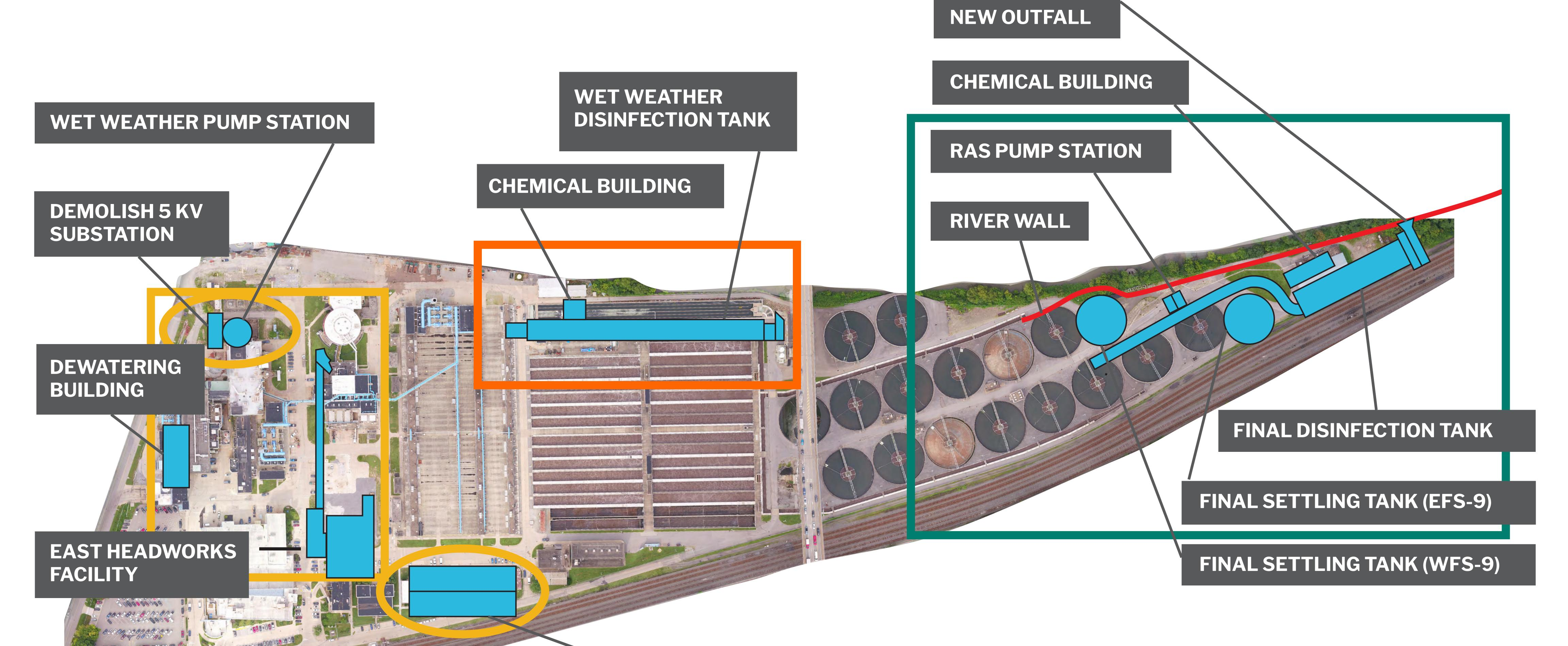
Expand Pumping, Headworks and Primary Capacity to 480 then to 600 MGD
