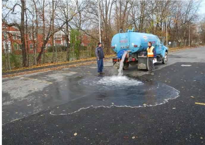
**Figure 2-13. Permeable Pavement Testing**
