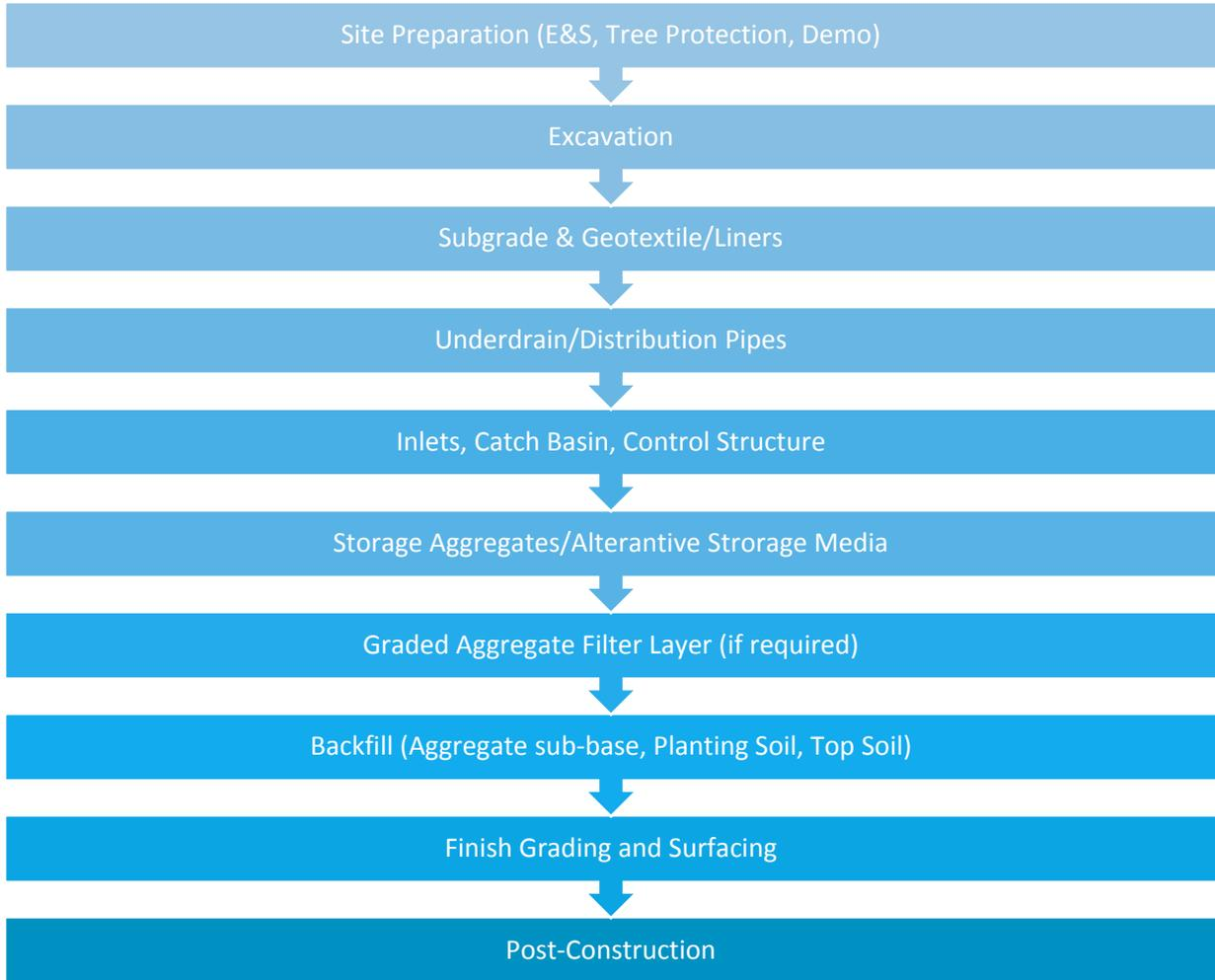
Figure 2-21. General Construction Sequence for Infiltration Trench Systems
