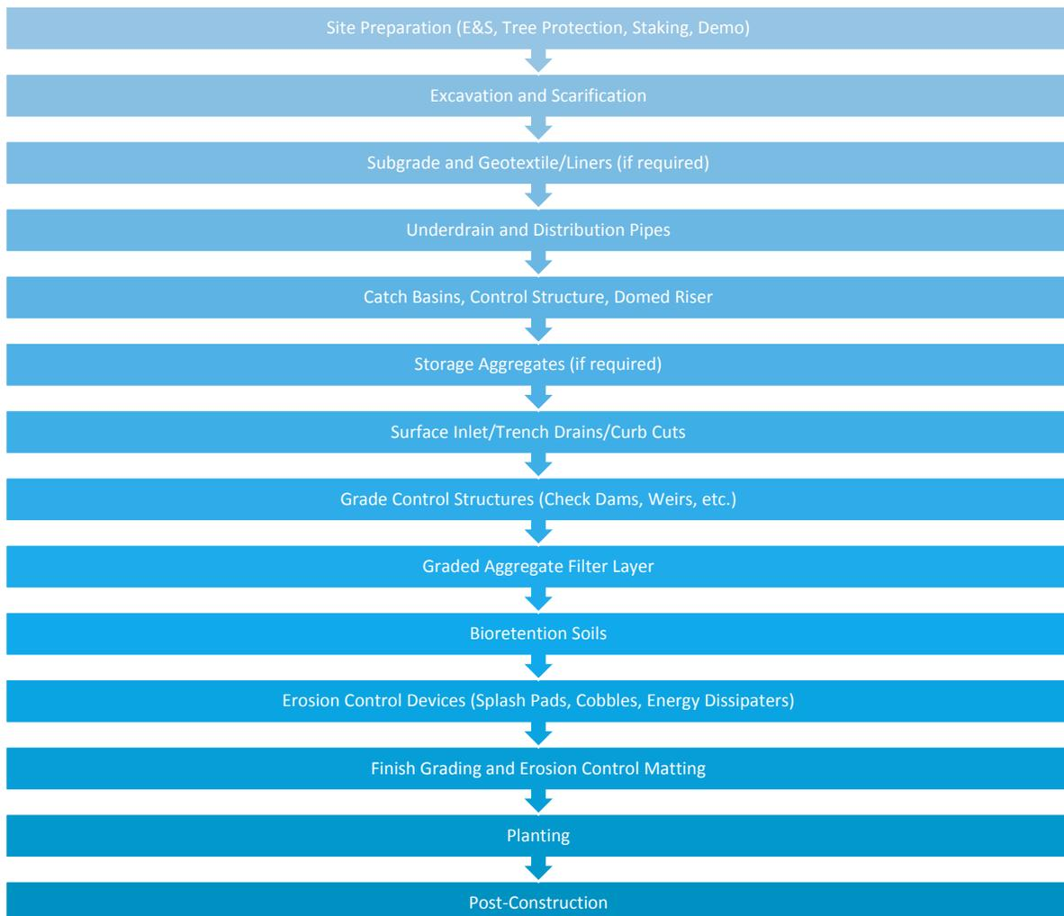
Figure 2-20. General Construction Sequence for Bioretention Systems
