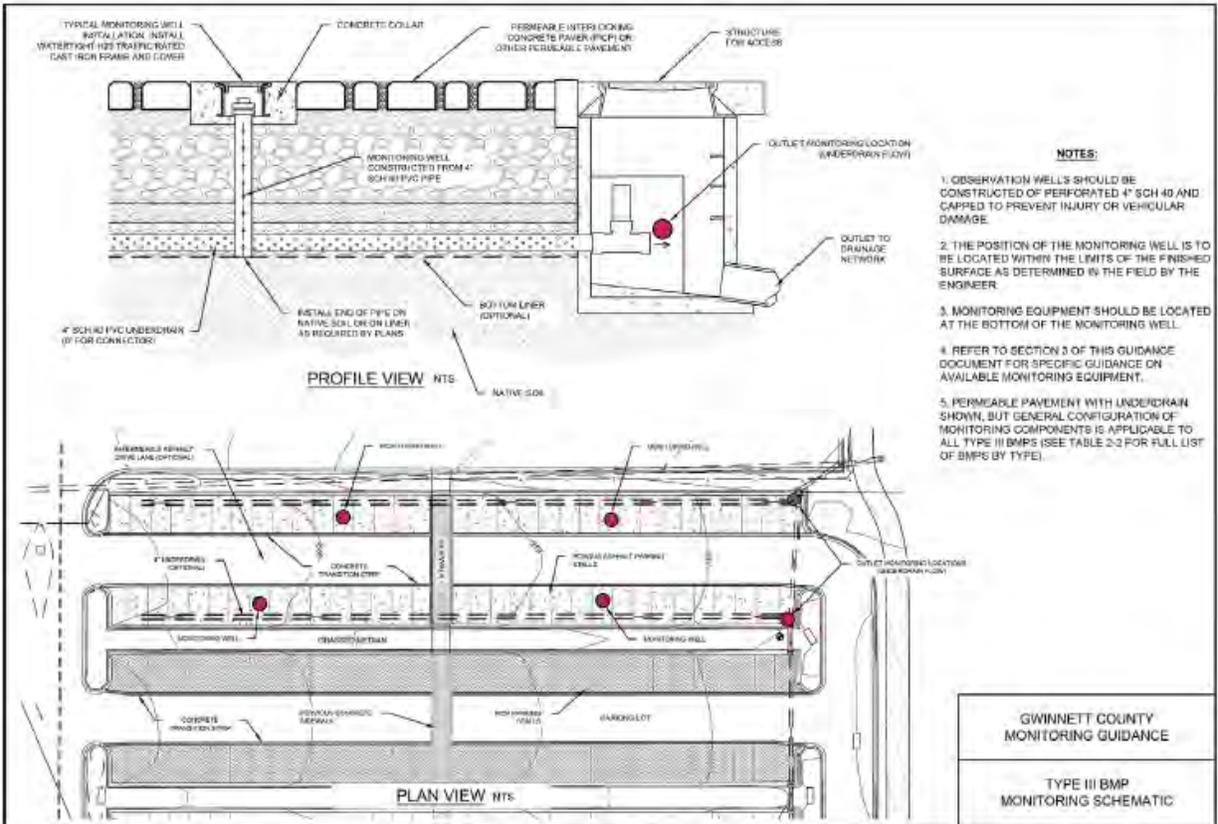
Figure 2-20. Example Schematic of a Permeable Pavement Site (Gwinnett County) In-GSI Monitoring Locations at the Outlet and Multiple Wells
