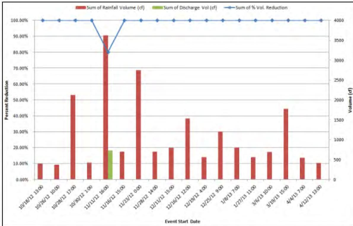
Figure 2-28. Rainfall volume, discharge volume, and percent volume reduction from a rain garden. Data recorded over a six-month period (Seattle Public Utilities)
