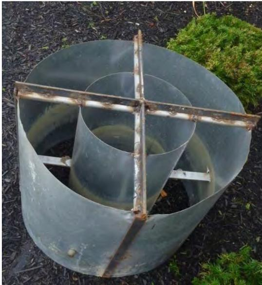
**Figure 2-23. GSI Infiltrometer Testing. (PWD)**
