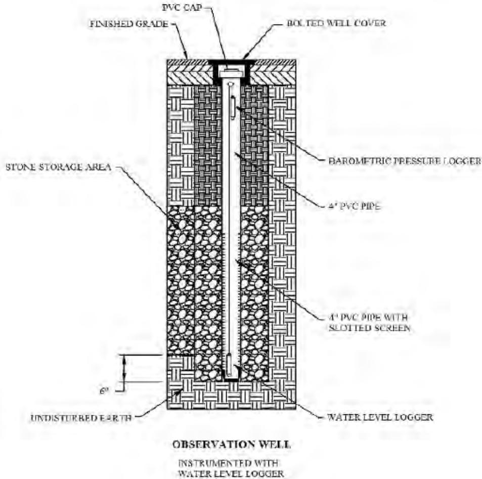
**Figure 2-17. Example Monitoring Well Schematic (PWD).**
