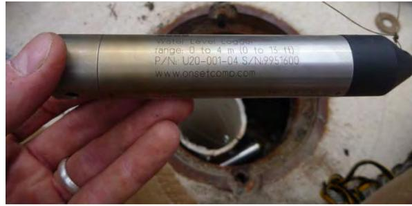
Figure 2-11. Onset HOBO Pressure Transducer (PWD)
