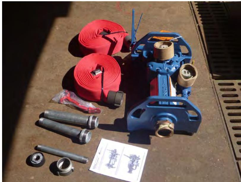
Figure 2-15. Simulated Runoff Test Equipment (PWD)
