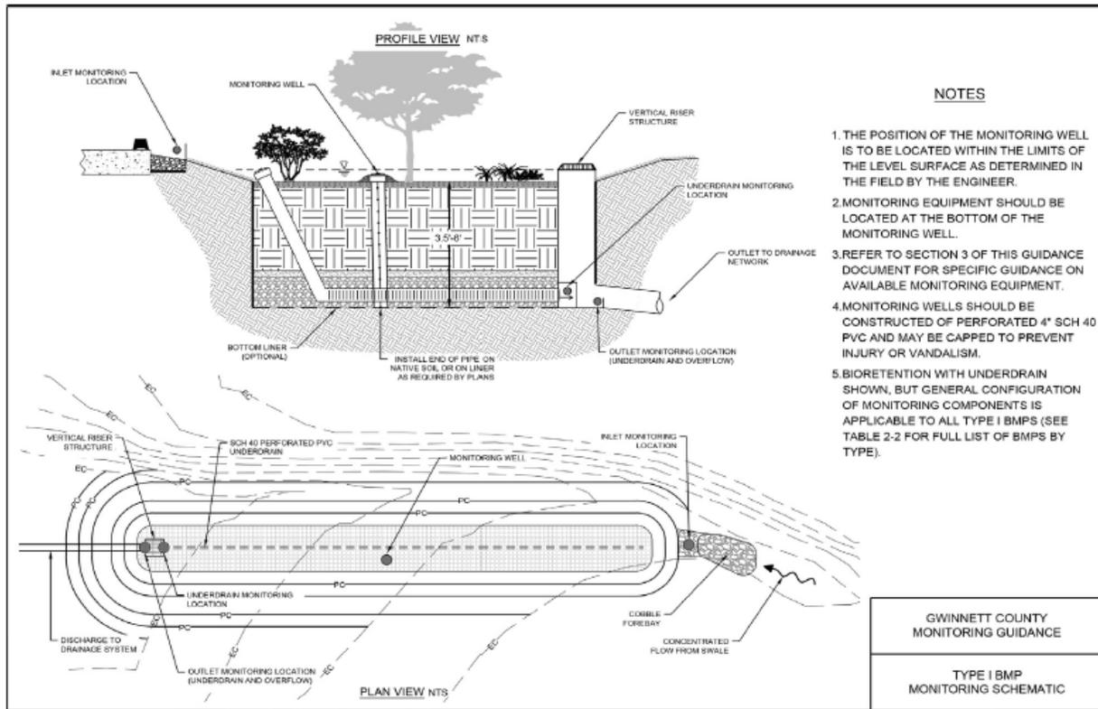
Figure 2-19. Example Schematic of a Bioretention Site (Gwinnett County) *In-GSI Monitoring Locations at the Inlet, Outlet, and Well*
