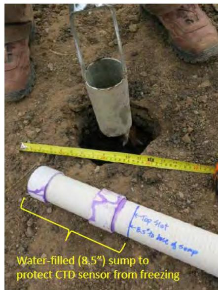
**Figure 2-24. Field measurement of sump depth**
