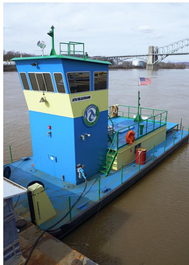
*Delivered in March, the 660hp "ATB Readshaw" gives ALCOSAN more power and maneuverability to maintain system structures inaccessible by land.*
